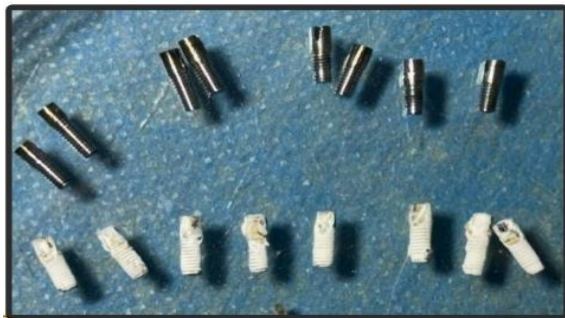
Figure 1: Uncoated versus nanocoated medical screws. While the length of each screw was 7 mm and diameter of the body was 2 mm.
